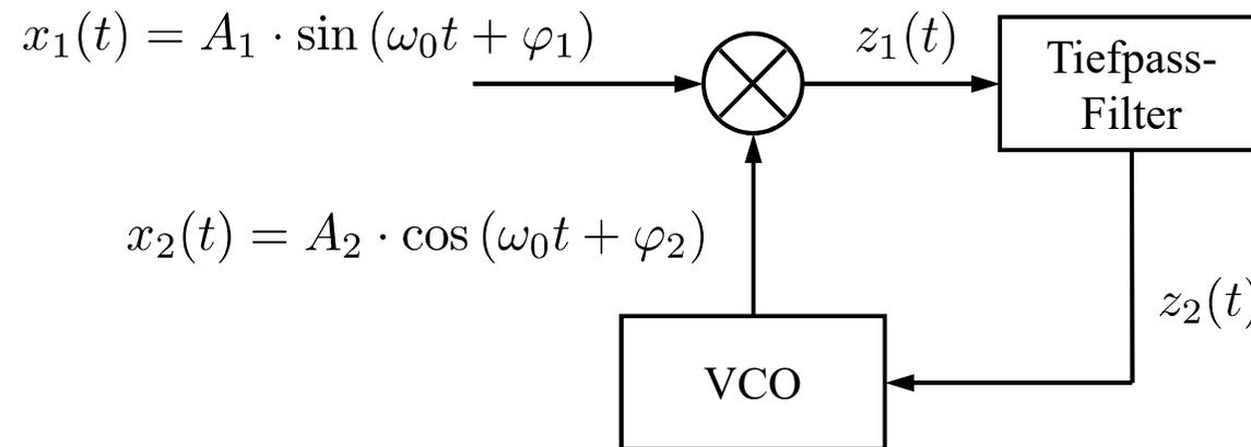
$$\begin{aligned} z_1(t) &= A_1 A_2 \cdot \sin(\omega_0 t + \varphi_1) \cdot \cos(\omega_0 t + \varphi_2) \\ &= \frac{A_1 A_2}{2} \cdot [\sin(\varphi_1 - \varphi_2) + \sin(2\omega_0 t + \varphi_1 + \varphi_2)] \end{aligned}$$
